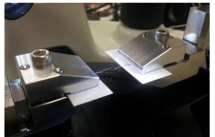
Once mounted in the UStretch test system, a test protocol with a 400mN preload and a constant velocity stretch of 15 $\mu$ m/s until failure was applied. Force/displacement data and time-correlated images were collected at 15Hz during the test.
