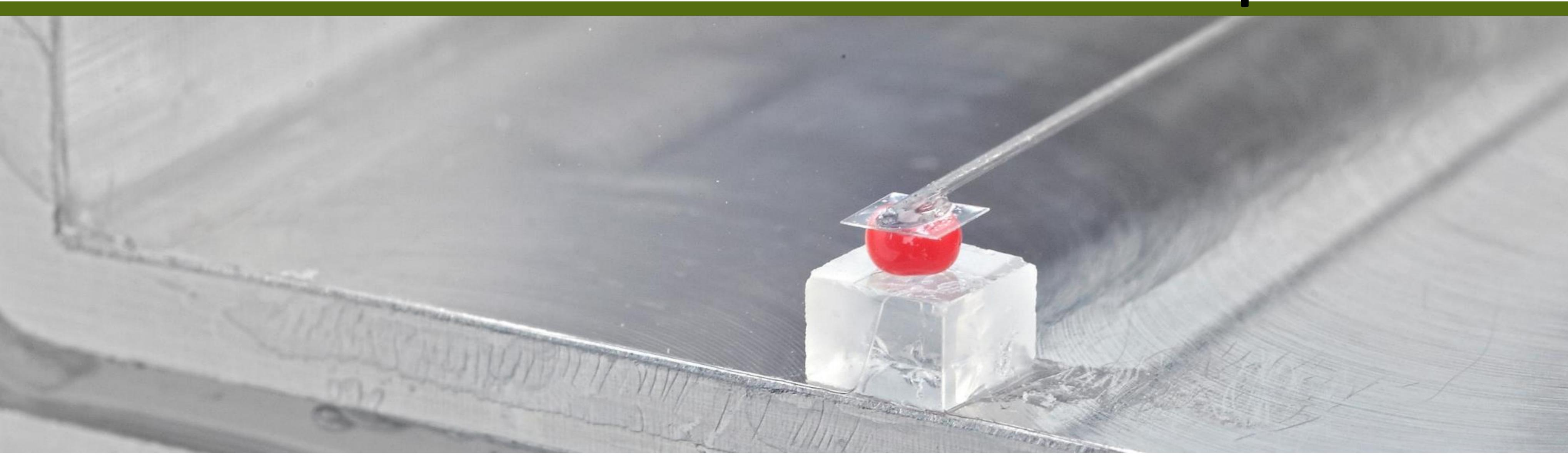
The MicroSquisher is a micro-scale tension-compression test system. It can be used to determine the stress-strain properties of a variety of materials including tissue samples, cell aggregates, hydrogels, and tissue engineering scaffold materials.
